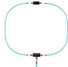
This simple, lightweight travel loop is quick to deploy and the perfect companion for Airspy and similar SDR radios!
