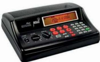
This 300-channel scanner can be categorized into 10 separate memory banks. Plus one-touch searches of marine, air and ham Frequency Range: 29-54 VHF Low Band. 87.3-107.9. 108-137 Civil Aircraft Band Includes 833 kHz steps. 137-144 VHF. 144-148 Amateur Band 2 Meters 148-174 VHF High Band
